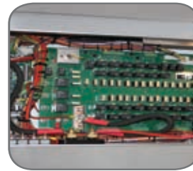
Printed Circuit Board with LED Diagnostic Lights
